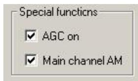
The AGC is turned off after the power on reset (POR) and can be
