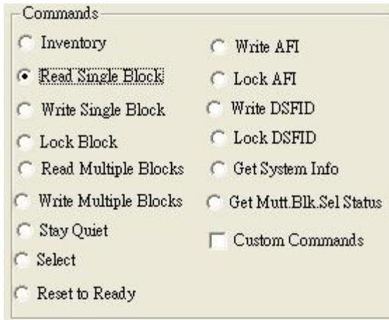
The Read Single Block command gets the data from one memory block of the responding tag. In addition to this data, a Block Security Status byte can be requested. This byte shows the write-protection of the block specified [e.g., unlocked, (user/factory) locked, etc.].
