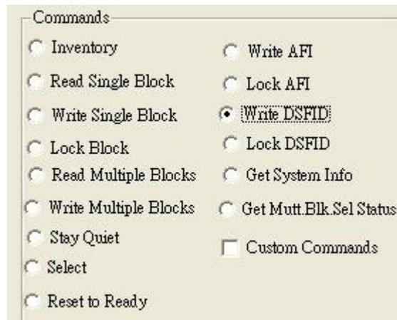
The *Write DSFID* (data storage format ID) command writes a new value in the DSFID register of the addressed tag(s). A corrupted response or lack of response does not necessarily indicate a failure to perform the write operation. Additionally, multiple transponders may process a nonaddressed request.
