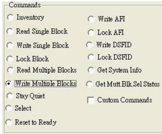
The *Write Multiple Blocks* command writes data to multiple memory blocks of the addressed tags. In order to successfully write data, the host must know the size of the memory block of the tag. *Write Multiple Blocks* is an optional command, and may not be supported by the tag (see the following screen capture).
